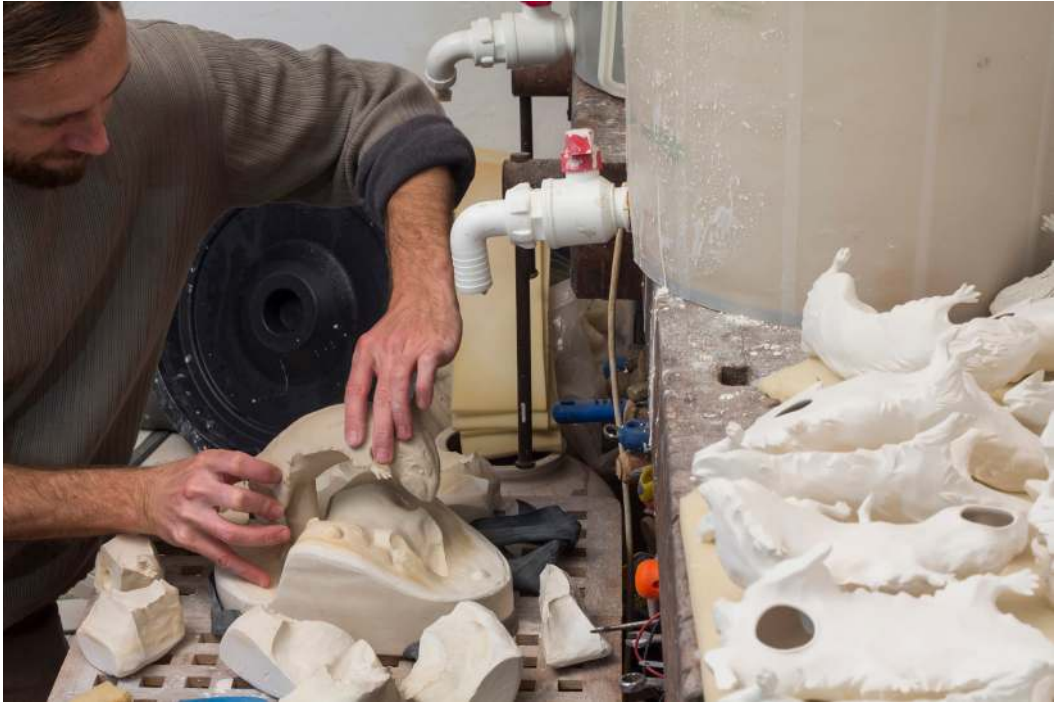
Removing the cast from the mould
